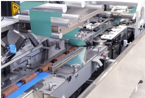
Image 1: Theegarten-Pactec has refined its FPC5 – a modular, high-speed packaging machine for wrapping chocolate bars in flow packs – to process paper-based packaging and recyclable mono-films.
