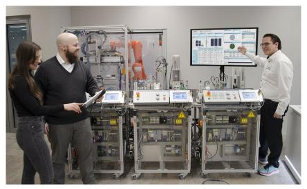
With the XITE Automax 600, Bosch Rexroth has developed a training system for both initial and further education, which brings abstract digitalization content to life and shows students the direct results of their work in a practical manufacturing context. (Image source: Bosch Rexroth AG)
