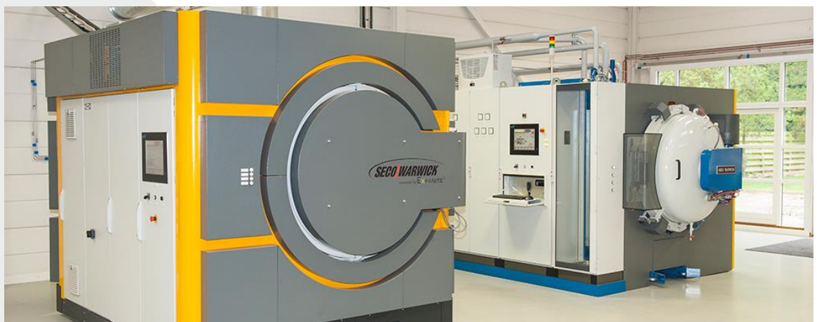
Photo 2: Furnaces for surface hardening stainless steel products
