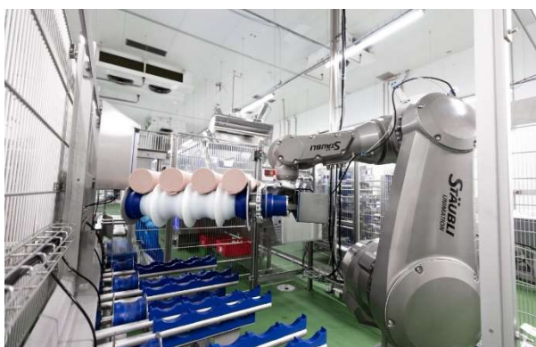
At Kaufland Fleischwaren, a TX200 HE has recently taken over the loading of an automatic slicing and packaging machine.
