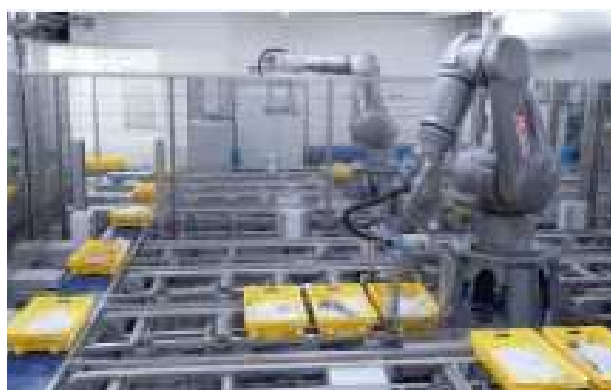
At the port of Guilvinec in Bretagne, TX200 HE six-axis robots handle containers filled with fresh fish.
