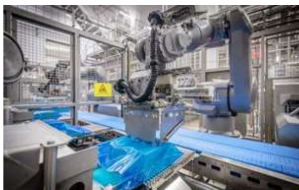
In hard cheese production at BMI Bayerische Milchindustrie eG, Stäubli HE robots take over the primary packaging of the freshly produced cheese blocks.
