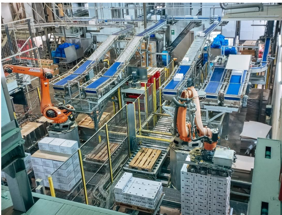
Caption: In the field of intralogistics, the leading supplier of frozen herbs relies on fully automated processes with two KUKA robots.
