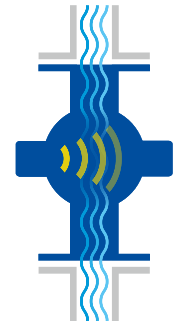
Schematic representation of a water/solids content measurement on a pipeline with FlowCell
