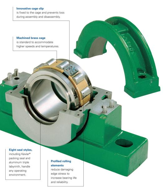
A split bearing can add value to your operations by significantly reducing downtime associated with moving equipment to change out a standard bearing. Easier to install, maintain and replace, split bearings can cut operational costs, free up your resources for other tasks and remove safety risk.
